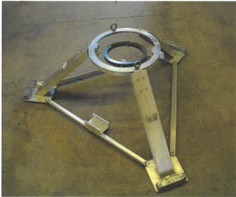
Photo of underwater mount for SonTek XR.
