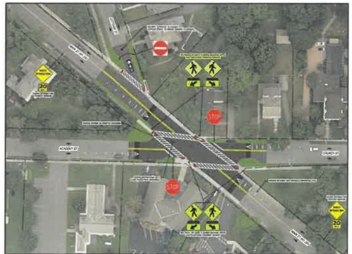
Figure 1: Intersection improvement concept for offset stop-controlled intersection in Greenwich, NY.
